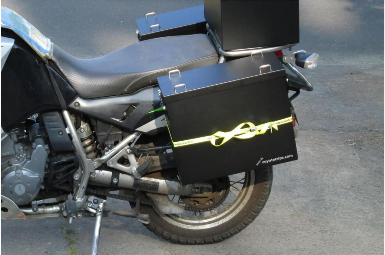
4. Attach the panniers to the racks using straps and move the panniers into a position that you like. Make sure that the panniers will not interfere with passenger footrests nor the maximum lean angle of the bike. Depending on the desired position of the panniers you might need to relocate the rear indicators. A relocating kit for the indicators may be supplied with your racks.
